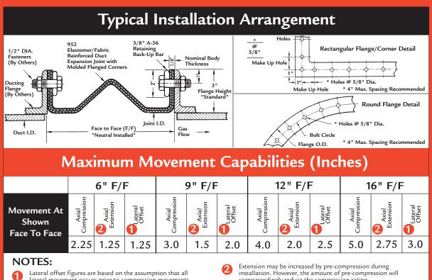
lateral movement occurs prior to compression movements. In practice, movements may occur simultaneously thus the allowable lateral offset may increase. Contact HÓLZ RUBBER for information.
