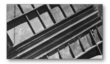
HOLZ RUBBER STYLE 952 ARCH-DESIGN EXPANSION JOINTS are designed for ultra-high movement in short face to face applications. Primarily for positive pressure clean systems having ultrahigh axial compression and extension movement, the Style 952 is constructed with a large, high, "V"-shaped arch which allows very high axial movement while exerting very low forces on the ductwork, duct flanges and equipment.
