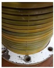
A Vibration dampening expansion joint installed within a mineral processing facility.
