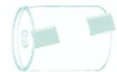
**Belt-Saver® Edge-Crown® protection pads** standard in 40 durometer industrial compound for use on non-drive pulleys in 10" lengths, formed to specific pulley diameters. Normally used in combination with Style 9 pads to provide a crown on flat face non-drive pulley. Available in the same compounds and backing plate combinations as Style 9 for special service conditions (Page 7). Bulletin PL 10877 A provides additional information on Style 11 Edge-Crown® pads.
