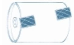
**Slide-Lag® Edge-Crown® traction pads** with standard 60 durometer industrial compound for use on drive pulleys, in 10" lengths, formed to specific pulley diameters. Normally used in combination with Style 5 pads to provide a crown on a flat face drive pulley. Also available in all special compounds and standard or stainless steel (SS) backing plates (Page 7). **NOW AVAILABLE IN “HUSKY”.**
