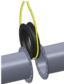
4. Install the flange bolts through the retaining rings, expansion joint and mating flanges from the arch side of the expansion joint. Metal washers are required at all splits of the retaining rings and are recommended on all bolts.
